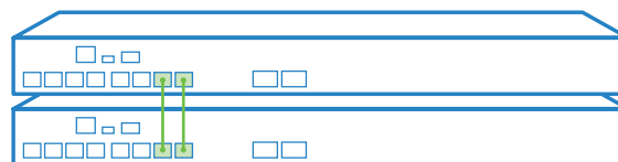
Fig. 12: Illustration of the cabling of a stack of 2 with the XS-5110F
