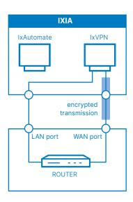
Figure 1: IXIA test system for routing connections and encrypted VPN connections between LAN and WAN
