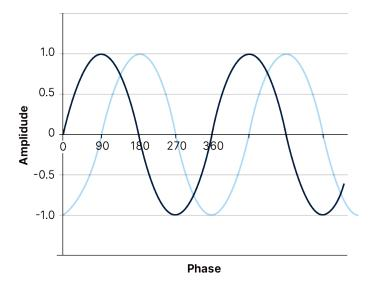
Figure 4: Both carriers of the QAM signal, same frequency, phase shifted by 90°
