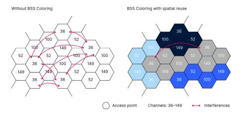
Figure 7: High interference without BSS Coloring and low interference with BSS Coloring and Spatial Re-Use
